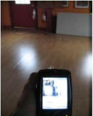
Whispy patterns characteristic of air infiltration are apparent at the periphery of the door trim. This is not a very large energy loss factor, but it can be a comfort factor and is easy to fix with caulk and / or paint. Also, as is the case with many of the exterior doors in this building, adjusting the striker place position slightly to compress the door gaskets can greatly reduce the air infiltration.
