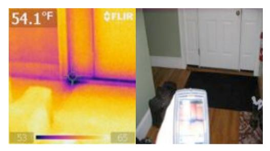
This image is of the front door, and illustrates a small amount of cool air leaking in the left corner of the front door, without the blower door operating, due to the force of stack effect. This airflow was perceptible with the back of the hand.
