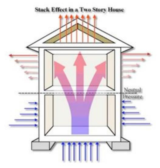
Note this is a heating season diagram, if the blue arrows indicate the direction and magnitude of the cold air pressure and direction entering the building, and the red arrows indicate the warmed air pressure and direction leaving the building.
