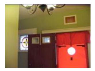
The blower door was installed in the front door. Air leakage (thin, whispy streams of dark cool air) are visible from behind the door above the left side lite trim. This is not a major cause of the high air infiltration, but is very easy to remedy with a bit of caulk.
